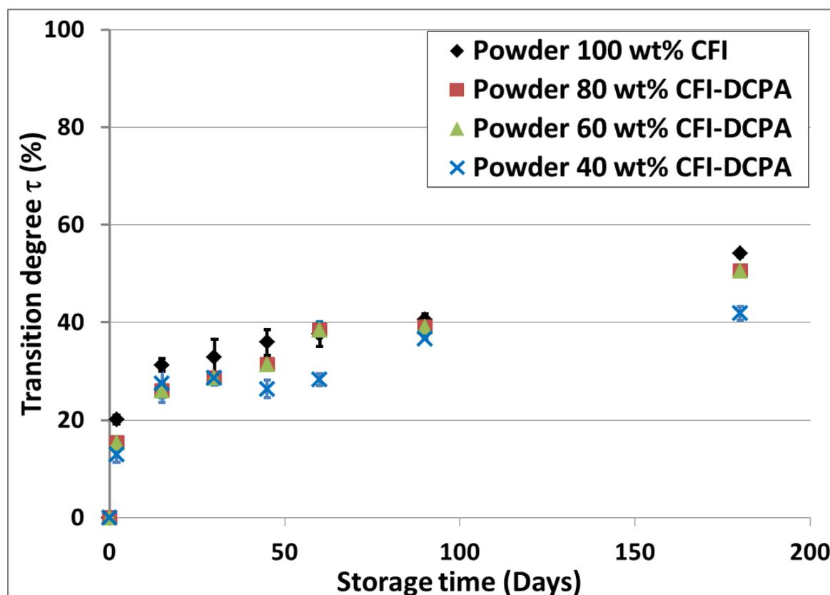
Fig.9: Evolution over time of the CFI transition degree in uncompressed powders for the four binary mixtures (CFI/DCPA), n=3.
