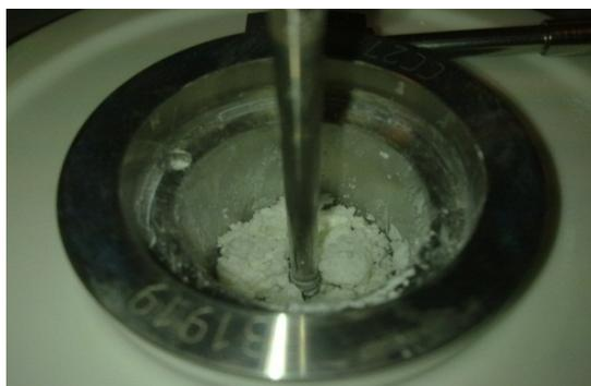
**Figure 8:** Formation of solid aggregates at 15% humidity, showing low viscosity
