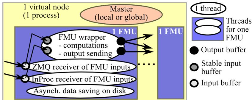
Figure 3: Multithreaded implementation of a virtual node
