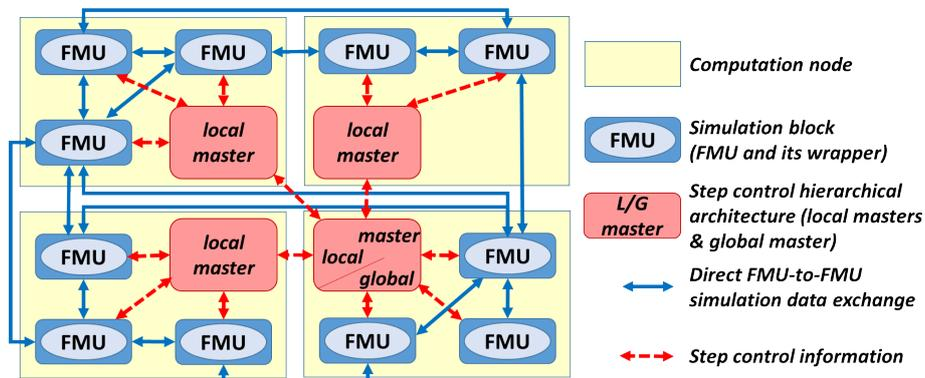
Figure 2: Distributed DACCOSIM architecture, with a hierarchical *master*
