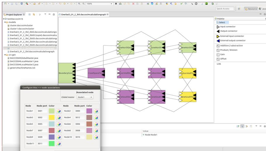
Figure 1: DACCOSIM GUI: FMU graph definition and configuration
