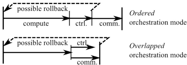
Figure 4: Two orchestration modes of a multi-simulation step
