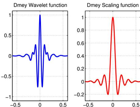
Figure 3: Dmey wavelet and scaling functions.
