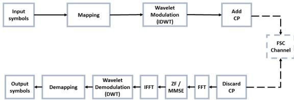
Figure 7: Wavelet transmission chain in a frequency selective channel.
