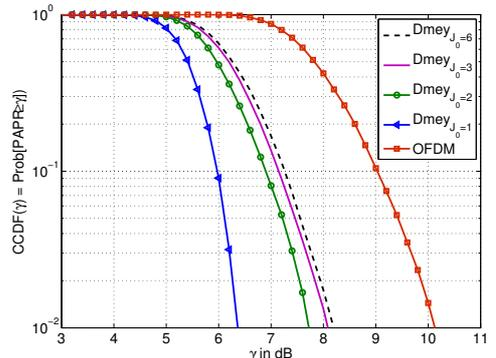
Figure 4: PAPR performance for different variants of Dmey wavelet.
