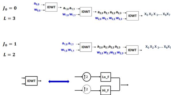
Figure 2: Wavelet-OFDM implementation for  $J_0 = 0$  and  $J_0 = 1$ .
