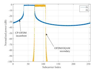
Fig. 2: Spectral representation of the Het scenario. CP-OFDM  $\mathcal{U}_1$  and OFDM/OQAM  $\mathcal{U}_2$  use directly adjacent bands  $\mathcal{L}_1$  and  $\mathcal{L}_2$  with same number of subcarriers.
