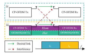
Fig. 1: Summary of the study led in the paper : two users  $\mathcal{U}_1$ and  $\mathcal{U}_2$  transmit on adjacent bands  $\mathcal{L}_1$  and  $\mathcal{L}_2$  and interfere with each other. Channel is assumed perfect and no Gaussian noise is considered.  $U_2$  uses CP-OFDM in *Hom* scenario and OFDM/OQAM in Het scenario.
