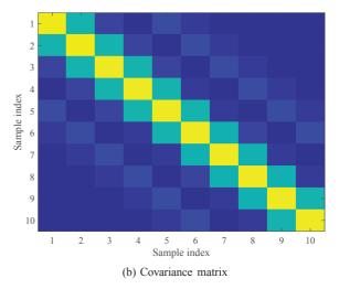
Fig. 6: Statistics of interference signal caused by OFDM/OQAM onto CP-OFDM subcarrier 72. The different results show that it can be modeled by a colored Gaussian noise.
