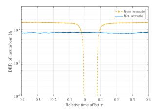
Fig. 9: Empirical BER of  $U_1$  versus the timing offset  $\tau$  between  $U_2$  and  $U_1$ , for *Het* and *Hom* scenarios.
