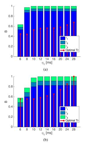
Fig. 1. Bandwidth optimal allocation minimising Trace (P) with respect to the randomly generated task set. The solid thick lines represent the normalised value of the traces. Results considering the presence of the delay (a) or not (b) are both reported for comparison.
