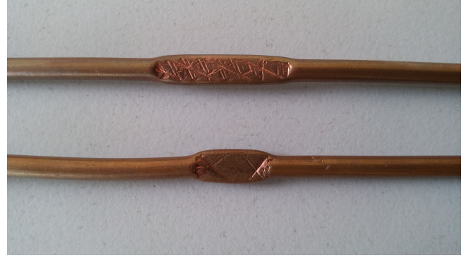
Fig. 2: The two faulty samples used to introduce soft faults within the NUTs for the experimental tests where the increasing the crushed area intensifies the reflection coefficient of the fault.
