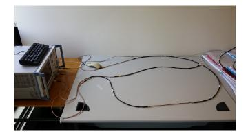
Fig. 3: Experimental setup for the single-junction NUT, containing two faulty sections, connected to the VNA for the experimental tests, schematized in Fig. 1(c).
