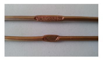
Fig. 2: The two faulty samples used to introduce soft faults within the NUTs for the experimental tests where the increasing the crushed area intensifies the reflection coefficient of the fault.
