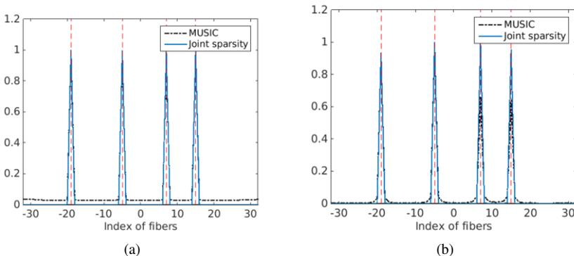
Figure 6. Imaging results of missing (a) carbon (b) glass fibers, with indices  $[-19, -5, 7, 15]$ ,  $N_r = N_s = 100$ ,  $f = 60\text{GHz}$ ,  $d = 0.1\text{mm}$ ,  $c = 0.2d$ ,  $\text{SNR} = 20\text{ dB}$
