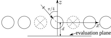
**Figure 3.** Validation by COMSOL with  $(-1)$ -th and  $1$ -th carbon fibers missing, incident wavelength  $\lambda^{inc} = d$ .
