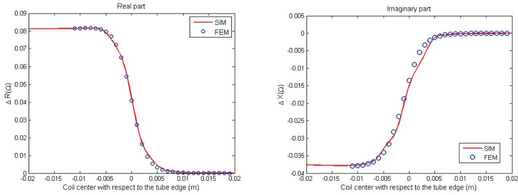
**Figure 3.** Comparison of the coil impedance variation of a tube with a crack at its edge as obtained from semi-analytical model following the SIM method with results obtained by COMSOL (FEM approach)
