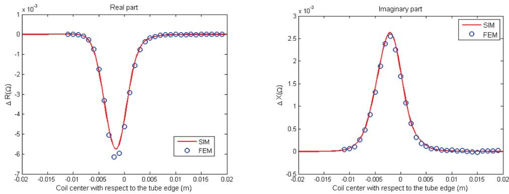
**Figure 4.** Contribution of the crack to the total signal as obtained from semi-analytical model following the SIM method with results obtained by COMSOL (FEM approach)
