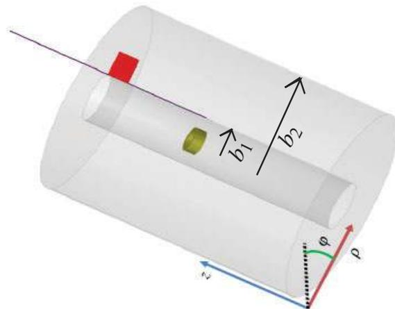
**Figure 1.** Inspection of a conducting tube of inner and outer radius  $b_1$  and  $b_2$ , respectively, with a crack at the edge of the tube. The flaw surface is on the  $\rho - z$  plane with a narrow azimuthal opening.
