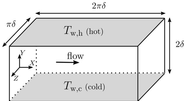
Figure 1: Channel flow configuration of half-width  $\delta$ . In heat transfer simulations, both wall temperatures  $T_{w,c}$  (lower wall) and  $T_{w,h}$  (upper wall) are prescribed where  $T_{w,h} \geq T_{w,c}$ .
