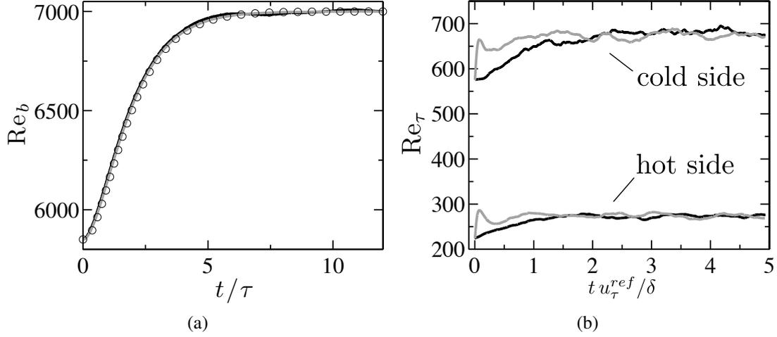
Figure 3: Temporal evolution of  $Re_b$  (a),  $Re_\tau$  on the cold and hot sides (b) for a non-isothermal case ( $T_{w,c}=950\text{K}, T_{w,h}=2050\text{K}$ ). Circles: theoretical solution; Black plain line:  $\tau = 0.33\delta/u_\tau^{ref}$ ; Gray plain line:  $\tau = 0.033\delta/u_\tau^{ref}$ .
