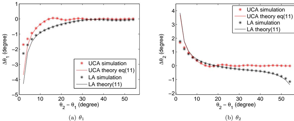
Figure 7: DOA estimation error vs. DOA separation (UCA with  $M = 20$ , LA with  $M = 20$  and  $d = \lambda/4$ , two sources with uniform angular dispersion,  $\Delta_0 = 10^\circ$ ,  $\theta_c = \frac{1}{2}(\theta_1 + \theta_2) = 60^\circ$ )
