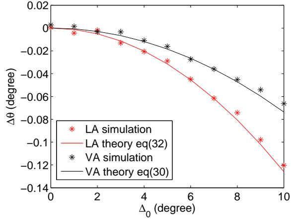
Figure 5: DOA estimation error vs. the source angular extension  $\Delta_0$  (LA with  $M = 20$  and  $d = \lambda/4$ , VA with  $M = 20$  and  $d = \lambda/4$  and  $\beta = 100^\circ$ , one source with uniform angular dispersion with  $\theta = 45^\circ$ ,  $\Delta_0 = 2\sqrt{3}\sigma$ )
