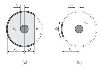
Fig. 7. Transversal cut of the coaxial line used in the numerical validation, with an internal conductor of radius  $r_i=0.5$  mm, external conductor of radius  $r_o=3$  mm, a dielectric with relative permittivity  $\epsilon_d=2.1$  (polytetrafluoroethylene, PTFE). The modified line is (a) partially cut along a distance D from its axis or (b) a simplified pigtail connection, where the external conductor is reduced to an angular region of 45 degrees, with the dielectric totally removed.
