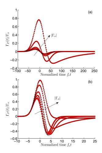
Fig. 4. Normalized time-domain echoes for an electrically-short fault, expected for a baseband Gaussian test signal with (a)  $B_o/f_c=0.01$  and (b)  $B_o/f_c=0.1$ . The different curves correspond to increasing values of  $\Gamma_o$  equal to 0.1, 0.2, 0.5, 0.7, 0.9 and 0.99, according to the direction of the arrows. Exact results (black solid lines) and approximations from the zero-pole model (red dots) are shown.
