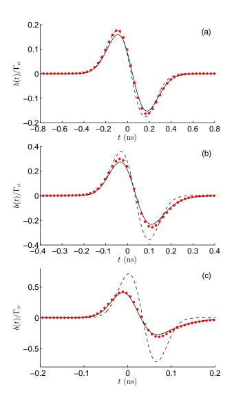
Fig. 9. Validation of the zero-pole model (9) and the derivative model (16), for the fault in Fig. 7(b) submitted to a Gaussian test signal with : (a)  $B_o = 1.25$  GHz, (b)  $B_o = 2.5$  GHz and(c)  $B_o = 5$  GHz. Numerical results are shown as red circles, predictions from the zero-pole model as solid black lines and for the derivative model as dashed lines. The critical frequency is  $f_o = 3.16$  GHz.
