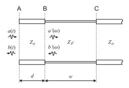
Fig. 1. Double impedance-step representation of a local fault in a transmission line of characteristic impedance  $Z_o$ , and relevant quantities for the derivation of the response  $\Gamma_F(\omega)$  of a fault of impedance  $Z_F$ .
