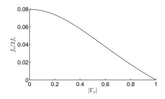
Fig. 6. Maximum normalized frequency  $f/f_c$  for which the derivative approximation holds, as a function of the fault severity  $|\Gamma_o|$ , evaluated taking a safety factor 2 below the frequency  $f_o/f_c$  in the condition (15).
