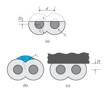
Fig. 10. Two-wire line with cylindrical conductors of radius  $r_i=0.5$  mm, a dielectric coating of thickness 1 mm ( $r_o=1.5$  mm) and relative dielectric constant  $\epsilon_d=3.5$  (polyvinyl chloride, PVC). The distance between the conductors axis is d=2 mm. The pictures illustrate the three faults considered: (a) a partial cut in the line; (b) the presence of a water droplet of radius  $r_w=2$  mm over the two conductors and c) a metallic slab partially inserted into the line.
