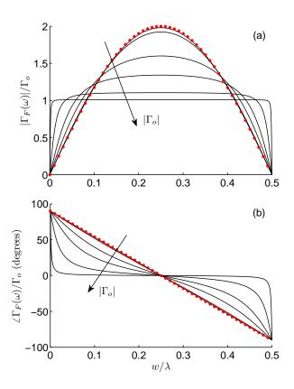
Fig. 2. Amplitude and phase-shift angle for the echo response  $\Gamma_F(\omega)$ predicted by (7), for six values of  $|\Gamma_o|$ , namely 0.1, 0.2, 0.5, 0.7, 0.9 and 0.99, in increasing order according to the direction of the arrows in the graphics. The red dots represent the soft-fault (weak perturbation) approximation (8).
