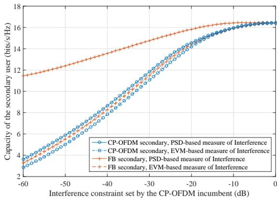
Fig. 6: Maximum capacity achieved by the secondary user with the PI-algorithm [10]. Gains obtained with the use of FB waveforms is significantly decreased when actual EVM values of interference are used instead of the flawed PSD-based approach.
