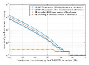
Fig. 5: Number of guard subcarriers necessary between the secondary and the incumbent as a function of the interference constraint set by the incumbent.
