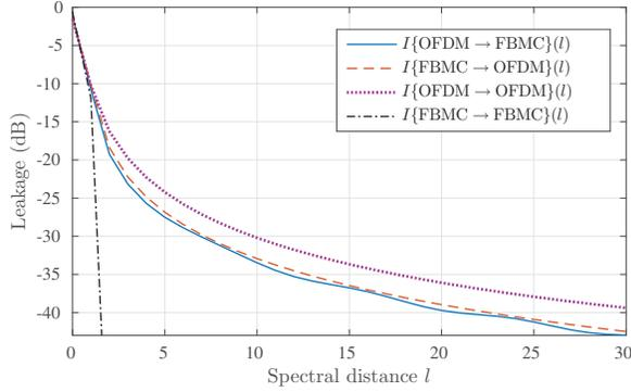
Fig. 2. Interference tables measuring the value of interference injected between different couples of waveforms according to [4]–[6].
