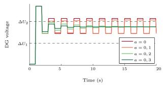
Fig. 5. Dynamical simulations of the voltage profile for a disturbance step with several rapidity filter settings
