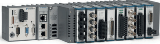
Fig. 6: Used NI multi-core cRIO-9082 platform.
