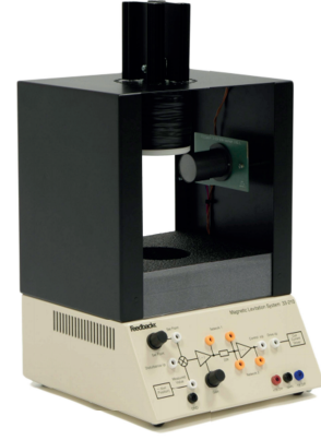
Fig. 7: Feedback MAGLEV 33-006 system.
