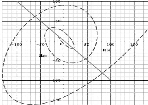
**Fig. 3** Bifurcations curves of (37) in the gains  $(a_{1,0}, a_{2,0})$  plan (solid red=Pitchfork singularity i.e. the zero singularity, discontinuous blue=Hopf singularity ) for the fixed value  $\tau_2 = \frac{7}{8}$ .
