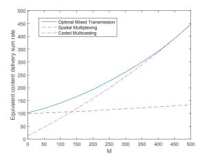
Fig. 2. The equivalent sum content delivery rate of optimal mixed transmission, spatial multiplexing and coded multicasting with user cache as a function of cache memory M for N = 2000, K = 100, P/K = 20 dB,  $\sigma^2 = \left(\frac{P}{K}\right)^{-1}$ .
