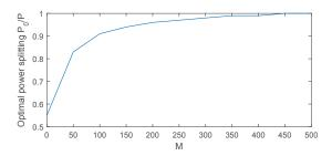
Fig. 3. The optimal power splitting, interpreted by the common power fraction  $P_0/P$ , as a function of cache memory M for N = 2000, K = 100, P/K = 20 dB,  $\sigma^2 = \left(\frac{P}{K}\right)^{-1}$ .
