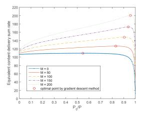
Fig. 1. The equivalent sum content delivery rate as a function of common signal power fraction  $P_0/P$ , and the optimal operating point computed by gradient descent method for N = 2000, K = 100, P/K = 20 dB,  $\sigma^2 = \left(\frac{P}{K}\right)^{-1}$ .
