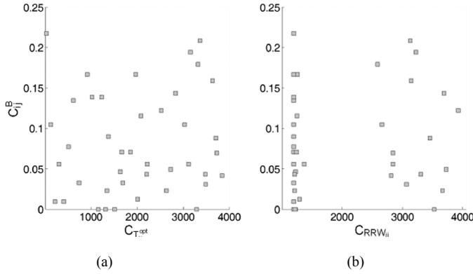
Fig. 10. Scatterplot of the Copeland scores of (a) the optimal repair time  $C_{T_{ij}}^{\text{opt}}$  and (b) resilience reduction worth  $C_{RRW_{ij}}$  with the shortest path betweenness  $C_{ij}^B$  for the links of the IEEE 30-bus network.
