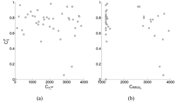
Fig. 11. Scatterplot of the Copeland scores of (a) the optimal repair time  $C_{T_{ij}}^{\text{opt}}$  and (b) resilience reduction worth  $C_{RRW_{ij}}$  with flow betweenness  $C_{ij}^F$  for the links of the IEEE 30-bus network.
