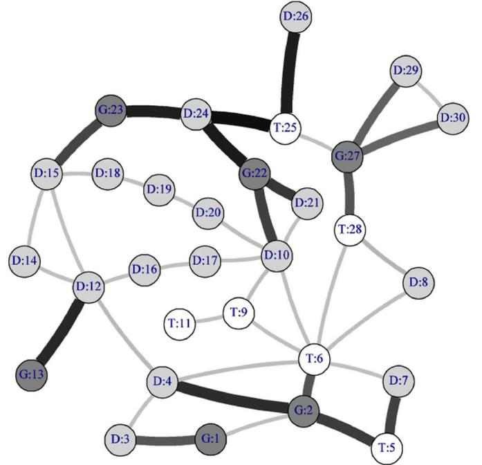
Fig. 9. Graphical illustration of the Copeland scores of the resilience reduction worth  $RRW_{ij}(\Delta t_0 = 3)$  for all IEEE 30-bus network links. Links with higher values of Copeland score are represented as thicker and darker edges.
