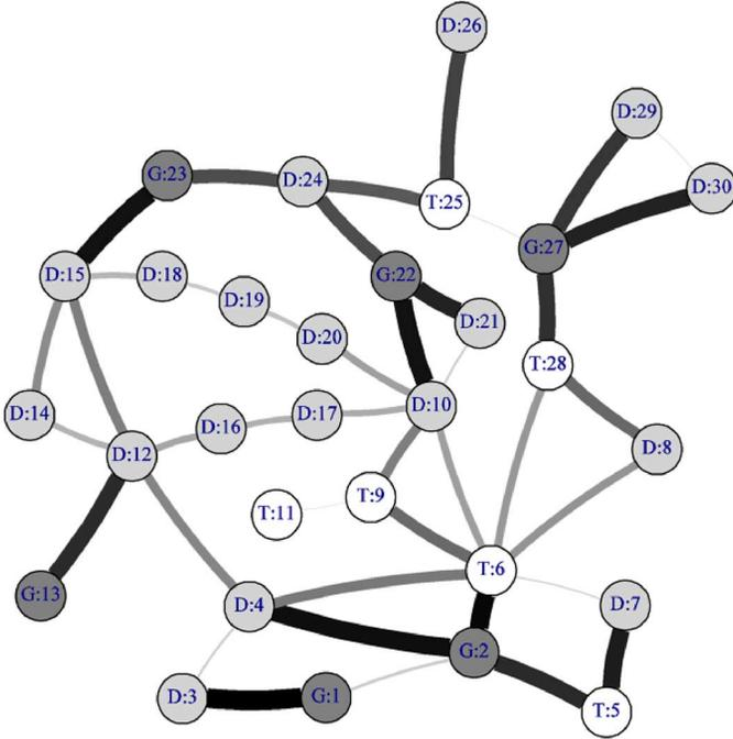
Fig. 7. Graphical illustration of the Copeland scores of the optimal repair time  $T_{ij}^{\text{opt}}$  for all IEEE 30-bus network links. Links with higher value of Copeland score are represented as thicker and darker edges.
