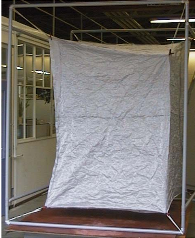
Fig. 12. The Vibrating Intrinsic Reverberation Chamber hanging on strings
