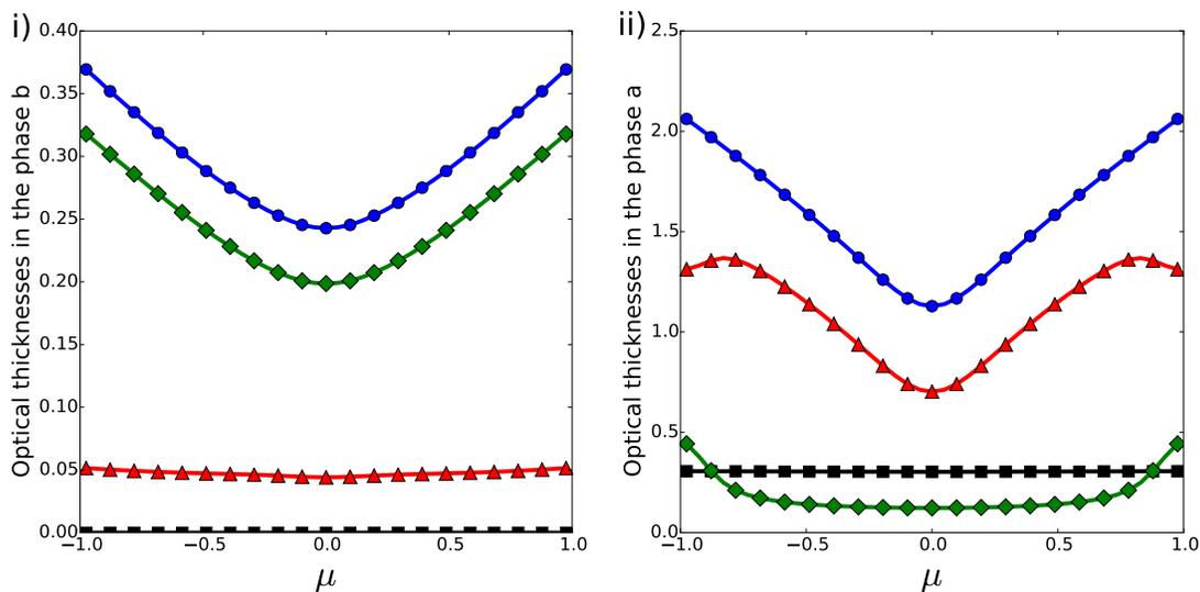
Figure 6: Optical thicknesses based on  $\circ$ : Generalised extinction coefficients ( $B_c d$ );  $\triangle$ : Generalised internal scattering coefficients ( $\Sigma_{cc} d$ );  $\diamond$ : Generalised external scattering coefficients ( $\Sigma_{cd} d$ ) and  $\square$ : Absorption coefficients ( $\kappa_a d = 0.3$  and  $\kappa_b d = 0$ );
