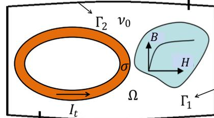
Fig. 1. Nonlinear electromagnetic problem coupled with electric circuits
