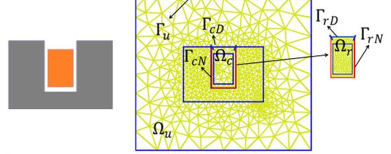
Fig. 2. Test-case example: solid conductor located in a lamination slot.
