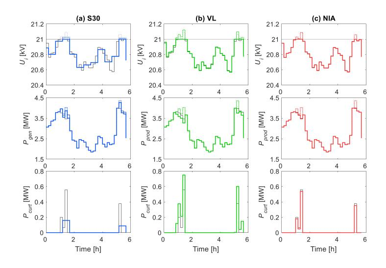
Fig. 5. Examples of voltage (top), generation power (middle) and curtailed power (bottom) computed by the exact load-flow solver (black lines on a, b and c), S30 (blue lines on a), VL (green lines on b), and NIA (red lines on c) before/after generation curtailment (dashed/solid lines).
