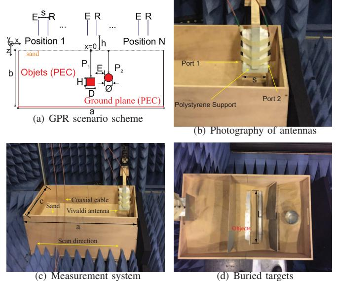
Fig. 1. GPR scenario scheme (a), the dimensions (in mm) being  $a = 1000$ ,  $b = 210$ ,  $c = 600$ ,  $H = 50$ ,  $D = 50$ ,  $L = 500$ ,  $P_1 = 125$ ,  $\phi = 50$ ,  $P_2 = 95$ ,  $E = 50$ ,  $S = 100$ ,  $h = 2$  and photos of the equipment (b) (c) (d).
