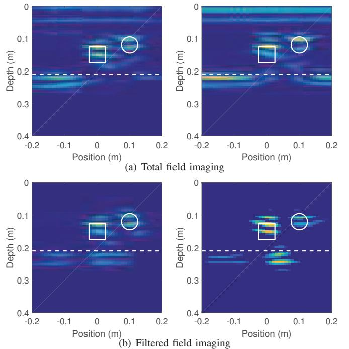
Fig. 3. KM imaging : CST-MWS (left) and measurement (right).
