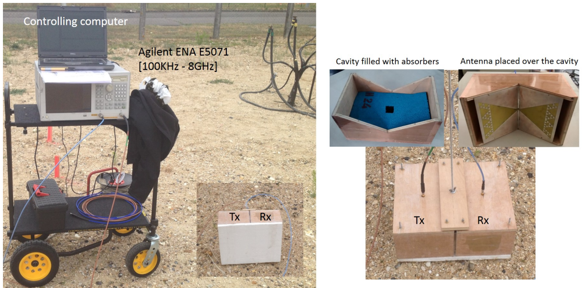
Figure 13: (left) Vector Network Analyzer and controlling computer, (right) transmitting and receiving antennas cavity backed V-folded bowtie antennas.
