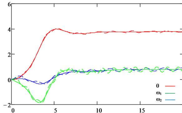
**Fig. 1** Simulation results for the system (9). The solid lines show the state trajectories for the case  $d_1(t) = d_2(t) = 0$ . The dashed lines correspond to the case  $d_1(t) = 0.8 \sin(3t)$ ,  $d_2(t) = 0.9 \sin(5t)$ .
