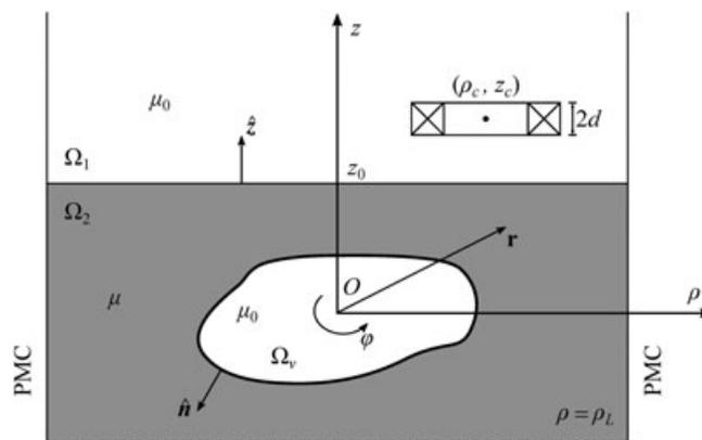
**FIGURE 1** Arbitrarily shaped air inclusion embedded within a conducting half-space, illuminated by a cylindrical coil. Lateral view with the cylindrical coordinate system of the truncated domain, using a perfect magnetic conductor (PMC) condition
