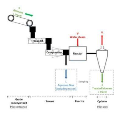
Fig. 1 - Process flow diagram of the pretreatment pilot.
