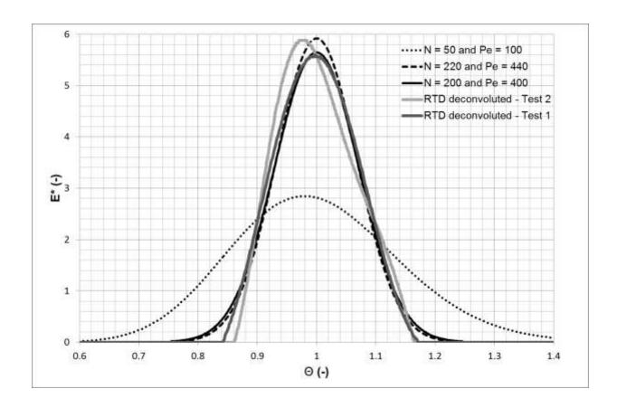
Fig. 9 - Comparison of the CSTR and ADM models with RTD curve- Test 1.
