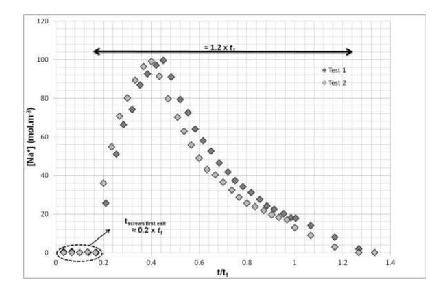
Fig. 4 - Na+ concentration in the aqueous flow as function of time - Tests 1 and 2.
