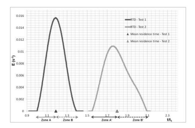
Fig. 7 - Residence time distributions for tests 1 and 2.
