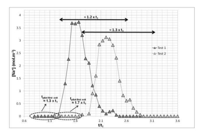
Fig. 3 - Na<sup>+</sup> concentration in the treated biomass - water solutions as function of time (samples collected at cyclone outlet) - Tests 1 and 2.
