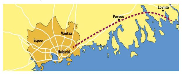
**Figure V-1:** Heat transportation system routing from the Loviisa 3 NDH unit to the Helsinki metropolitan area, about 80 km long. Data sources: ISNP, 2014.
