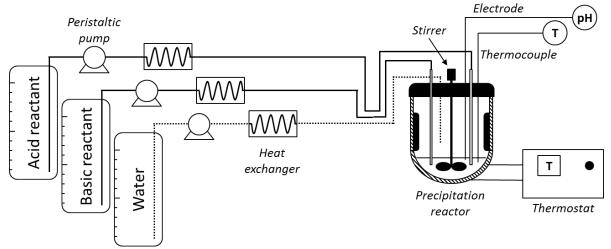
**Figure 1.** Schematic view of the experimental setup.
