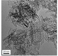
Figure 10. TEM image of  $\gamma$ -alumina A-500.
