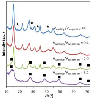
**Figure 2.** Evolution of the crystallographic phases in AACH cake with increasing washing volumes (secondary phases: ammonium nitrate ( $\star$ ); boehmite ( $\blacksquare$ )).
