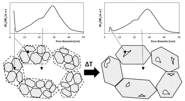
**Figure 13.** Schematic representation of the sintering phenomenon of AACH-derived alumina intracrystalline porosity between 500  $^{\circ}$ C and 700  $^{\circ}$ C.
