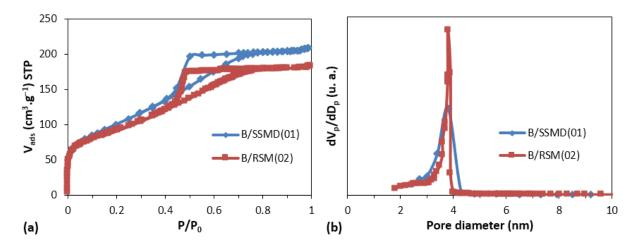
Figure 5. N<sub>2</sub> adsorption-desorption isotherms (a) and pore size distributions (b) of boehmite obtained by precipitation in fast contacting mixers SSMD and RSM.
