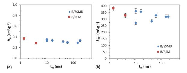
Figure 7. Pore volume (a) and specific surface area (b) evolution with micromixing time of boehmite precipitated in SSMD and RSM.
