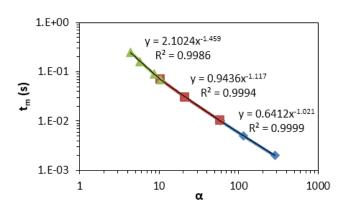
Figure 2. Micromixing time  $t_m$  against micromixedness ratio  $\alpha$ .
