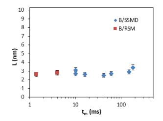
Figure 6. Average crystallite size evolution with micromixing time of boehmite precipitated in SSMD and RSM.
