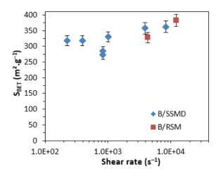
Figure 8. Specific surface area evolution with the shear rate of boehmite precipitated in SSMD and RSM.
