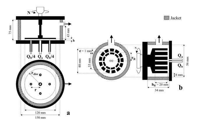
Figure 1. Schematic representation of investigated fast contacting mixers: front and bottom views of the SSMD (a), and front and profile views of the RSM (b).
