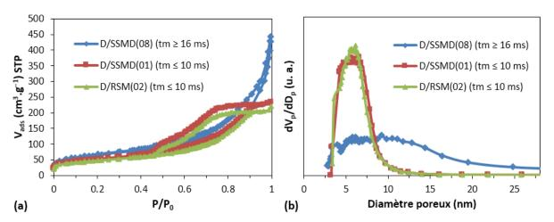
**Figure 9.** N<sub>2</sub> adsorption-desorption isotherms (a) and pore size distributions (b) of NH<sub>4</sub>-dawsonite obtained by precipitation in fast contacting mixers SSMD and RDT.
