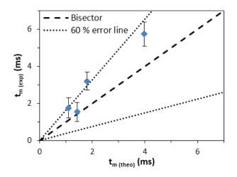
Figure 4. Experimental micromixing time against theoretical micromixing time (RSM).
