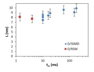
Figure 10. Average crystallite size evolution with micromixing time of NH<sub>4</sub>-dawsonite precipitated in SSMD and RSM.
