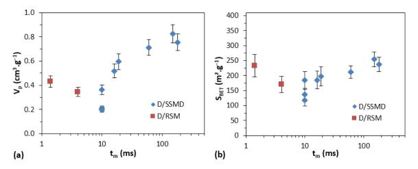
Figure 11. Pore volume (a) and specific surface area (b) evolution with micromixing time of NH<sub>4</sub>-dawsonite precipitated in SSMD and RSM.
