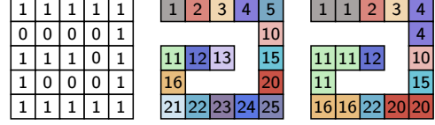
Fig. 7. From left to right: binary image, DLP-I labels initialization (with e_{(i,j)} = i \times 5 + j + 1 ) and first DLP-SR iteration with the 2 \times 2 mask.
