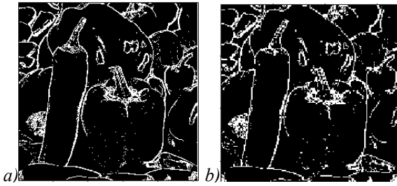
Fig. 2. Results of (a) classic convolution by a Sobel kernel (equivalent to 1 PE per pixel) and (b) down-sampled convolution with same kernel (equivalent to 1 PE per 9 pixels), performed on the classic image of peppers (512x512 pixels result in (b) 170x170 pixels).
