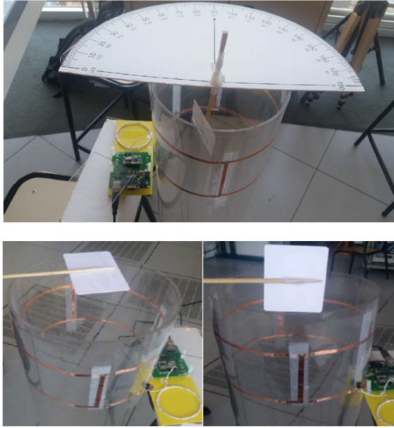
Fig. 8 Realized 3D design [13] with the tag inside the tube (top), parallel to the tube section (bottom left), and perpendicular to the edges of the tube (bottom right)
