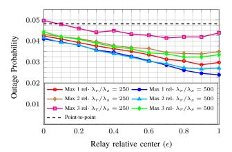
Fig. 9. Outage probability for NNC as a function point around which the relays are chosen, one the line between source and destination, for different relative densities.  $P_r/P_s = -10 \text{dB}$ ,  $\lambda_s = 10^{-4}$ , R = 1 b/use,  $\alpha = 4$ . d = 10. OP is optimized w.r.t. the noise compression variance.
