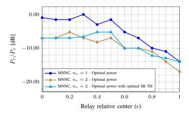
Fig. 12. Optimal power for MNNC corresponding to the OP of Fig. 11. Using more than one relay allows the reduction of the relay power.  $\lambda_r/\lambda_s = 500$ ,  $\lambda_s = 10^{-4}$ , R = 1b/use,  $\alpha = 4$ .
