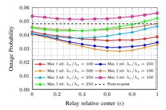
Fig. 8. Outage probability for ODF as a function point around which the relays are chosen, one the line between source and destination, for different relative densities.  $P_r/P_s = -10 \text{dB}$ ,  $\lambda_s = 10^{-4}$ , R = 1 b/use,  $\alpha = 4$ .
