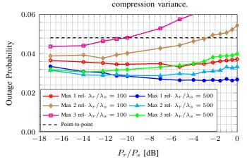
Fig. 7. Outage probability for MNNC as a function of the relative transmission power between relays and sources, for different relative densities.  $P_r/P_s=-10dB$ .  $\lambda_s=10^{-4}$ , R=1b/use,  $\alpha=4$ . Relays are chosen centered around the midpoint between a source and its destination ( $\epsilon=0.5$ ). The OP is optimized w.r.t. the noise compression variance.
