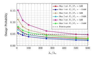
Fig. 3. Outage probability for NNC as a function of the relative density between relays and sources, for different relay-source relative transmission powers.  $\lambda_s = 10^{-4}$ , R = 1b/use,  $\alpha = 4$ . Relays are chosen centered around the destination ( $\epsilon = 1$ ). OP is optimized w.r.t. the noise compression variance.
