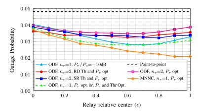
Fig. 13. Outage probability for ODF with optimized relay power and thresholds, compared to the best performance obtained with MNNC.  $\lambda_r/\lambda_s = 500$ ,  $\lambda_s = 10^{-4}$ , R = 1b/use,  $\alpha = 4$ .
