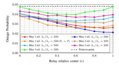
Fig. 10. Outage probability for MNNC as a function point around which the relays are chosen, one the line between source and destination, for different relative densities.  $P_r/P_s = -10 \text{dB}$ ,  $\lambda_s = 10^{-4}$ , R = 1 b/use,  $\alpha = 4$ . OP is optimized w.r.t. the noise compression variance.
