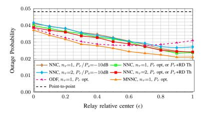
Fig. 14. Outage probability for NNC with optimized relay power and thresholds, compared to the best performance obtained with MNNC and ODF.  $\lambda_r/\lambda_s = 500$ ,  $\lambda_s = 10^{-4}$ , R = 1b/use,  $\alpha = 4$ . OP is optimized w.r.t. the noise compression variance.
