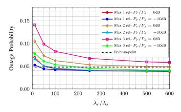
Fig. 2. Outage probability for ODF as a function of the relative density between relays and sources, for different relay-source relative transmission powers.  $\lambda_s = 10^{-4}$ , R = 1b/use,  $\alpha = 4$ . Relays are chosen centered around the source ( $\epsilon = 0$ ).
