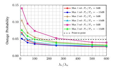
Fig. 4. Outage probability for MNNC as a function of the relative transmission power between relays and sources, for different relative densities.  $\lambda_s = 10^{-4}$ , R = 1b/use,  $\alpha = 4$ . Relays are chosen centered around the midpoint between a source and its destination ( $\epsilon = 0.5$ ). The OP is optimized w.r.t. the noise compression variance.
