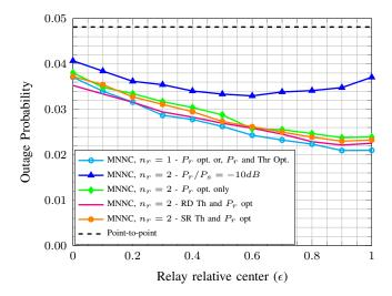
Fig. 11. Outage probability for MNNC with optimized relay power and thresholds.  $\lambda_r/\lambda_s = 500$ ,  $\lambda_s = 10^{-4}$ , R = 1b/use,  $\alpha = 4$ .
