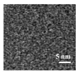
Fig. 4. HRTEM image of GaP grown at 380 °C with constant RF power (20 W) mode. Several examples of GaP ordered areas are marked by dot contours.
