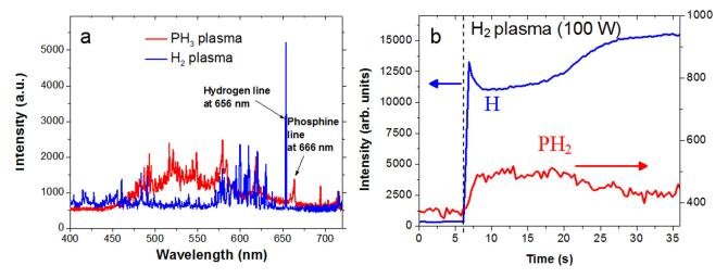
Fig. 9. (Color online) OES spectra of  $H_2$  and  $PH_3$  plasma (a). Time dependence of  $H_2$  (656 nm) and  $PH_2$  (666 nm) OES lines for  $H_2$  plasma treatment after P deposition during 30 s (b).
