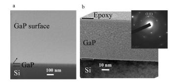
Fig. 1. SEM  $20^\circ$  tilt (a) and TEM bright field (b) cross section images of the GaP film grown on Si at  $380\,^\circ$ C with constant RF power (20 W) mode. SAED pattern by TEM is presented in the inset.
