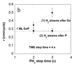
Fig. 8. Deposition rate (r) as a function of TMG (a) and PH<sub>3</sub> (b) deposition step time for GaP deposited with pulsed RF power (100 W) using H<sub>2</sub> plasma treatment after Ga deposition step (1) and H<sub>2</sub> plasma treatment after P deposition step. PH<sub>3</sub> (a) and TMG (b) deposition step times were fixed to 2 and 4 s, respectively. The level of one GaP monolayer (ML) is also indicated.
