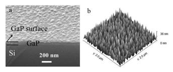
Fig. 7. SEM 20° tilt cross section image (a) and surface morphology by AFM (b) for GaP grown on Si with pulsed RF power (100 W) during deposition steps.
