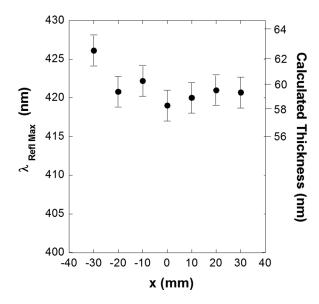
Fig. 11. Wavelength of the reflection maximum ( $\lambda_{Refl\ Max}$ ) vs distance for 3 in. Si substrates with GaP film deposited with H<sub>2</sub> plasma treatment step after P deposition step. Calculated GaP film thickness, which corresponds to  $\lambda_{Refl\ Max}$ , is indicated on the left axis.
