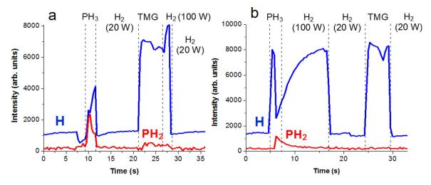
Fig. 10. (Color online) Time dependence of  $H_{\alpha}$  (656 nm) and  $PH_2$  (666 nm) OES lines for the processes with  $H_2$  plasma treatment step after Ga deposition step (a) and after P deposition step (b).
