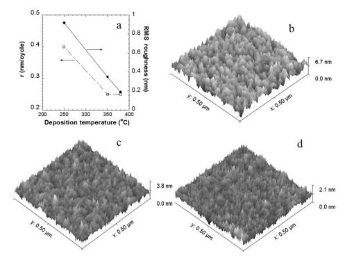
Fig. 2. Temperature dependence of the deposition rate (r) and RMS roughness (a) and surface topology by AFM for GaP deposited at  $250\,^{\circ}$ C (b),  $350\,^{\circ}$ C (c), and  $380\,^{\circ}$ C (d).
