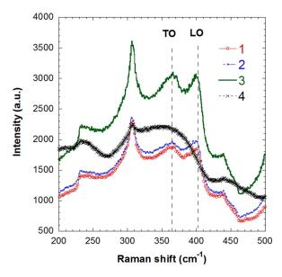
Fig. 5. (Color online) Raman spectra of GaP deposited on Si with pulsed RF power (100 W) during Ga and P deposition steps: without  $\rm H_2$  plasma treatment (1), with  $\rm H_2$  plasma (100 W) treatment step after Ga and P deposition steps (2), with  $\rm H_2$  plasma (100 W) treatment step after P deposition step only (3). GaP deposited at low RF power (20 W) during Ga and P deposition steps but with  $\rm H_2$  plasma (100 W) treatment step after Ga and P deposition step (4).
