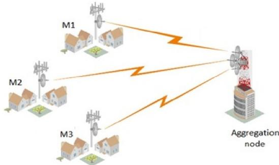
Figure 1: Backhaul network. The aggregation node handles all the traffic produced by and to nodes M1, M2, M3.
