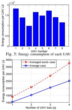
Fig. 6: Energy consumption vs. number of battery depleted UAVs.
