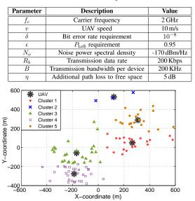
Fig. 2: Optimal clusters and UAVs' locations in one snapshot.
