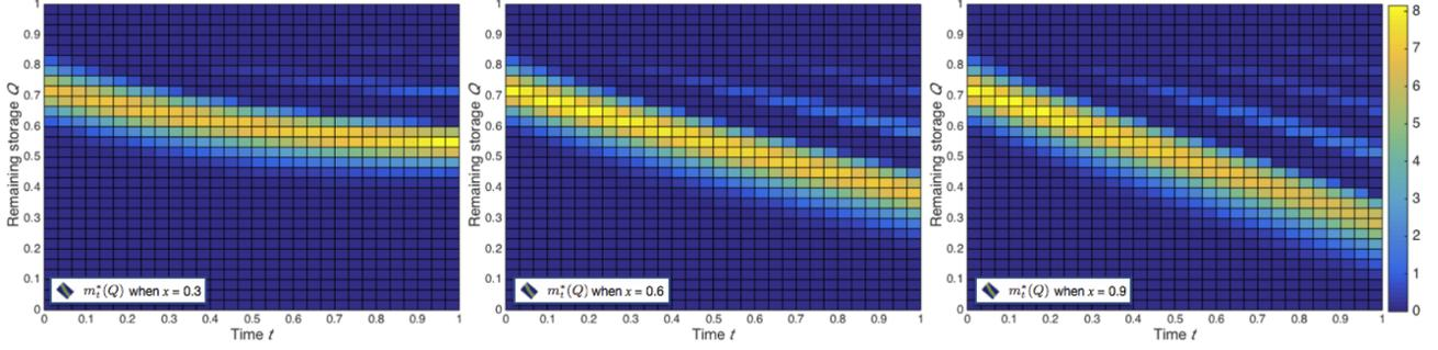
Fig. 4: Evolution of the MF distribution  $m_t^*(Q)$  that indicates the density of SBSs having the remaining storage space  $Q$  at time  $t$  with respect to different content popularity  $x$ ,  $B = 1$ ,  $N_{r(j)} = 20$ ,  $\mu = 0.1$ ,  $\lambda_u = 0.001$ ,  $\lambda_b = 0.03$ ,  $R = 10/\sqrt{\pi}$ .
