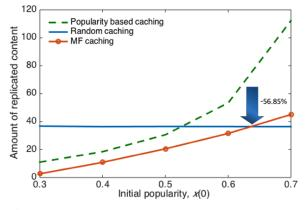
Fig. 6: The amount of replicated contents per storage usage ( $Q(0) = 0.7, \eta = 0.1, a = 0.15, u = 0.1$ ).
