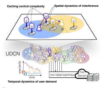
Fig. 1: An illustration of ultra-dense edge caching networks (UD-CNs) with spatio-temproal user demand and network dynamics.
