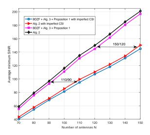
Fig. 7: Evaluating the impact of imperfect CSI at the BS for the MMF Problem with G=4,  $K_j=15 \ \forall j$  and P=10 Watt. Channel estimation is performed using an MMSE estimator that exploit UL pilot signals of length  $\tau_p=K$  and power equal to 1 Watt.
