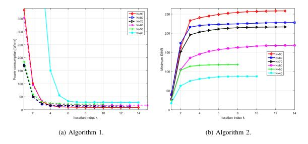
Fig. 6: The convergence behavior of Algorithms 1 and 2 for different number of antennas N.
