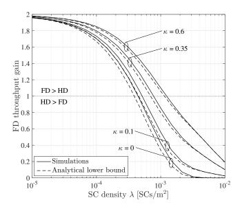
Figure 3. The impact of SC density  $\lambda$  on the FD throughput gain.
