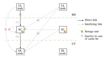
Figure 1. System model with cache-aided SCs, UL nodes, and DL nodes, with corresponding direct and interfering links.
