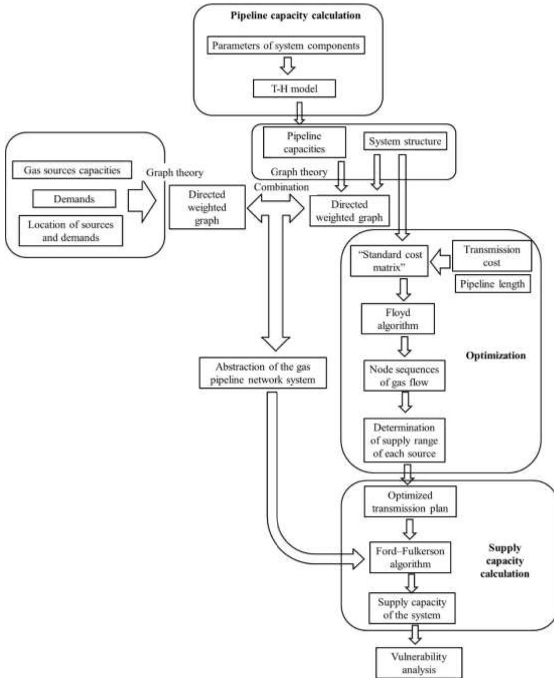
Fig. 2 Flowchart of the capacity/consequence analysis model
