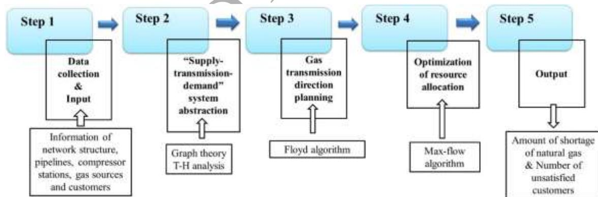
Fig. 1 Process of modeling for consequence analysis
