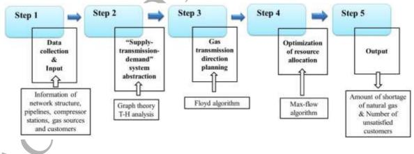
Fig. 1 Process of modeling for consequence analysis
