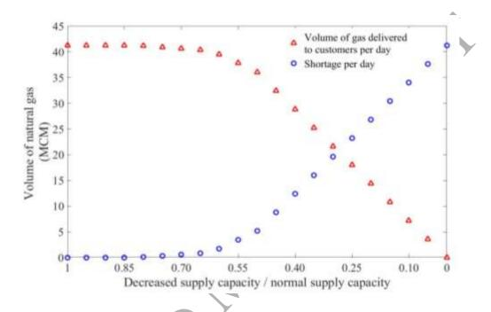
Fig.7. Global vulnerability analysis based on degeneration of supply capacities of sources
