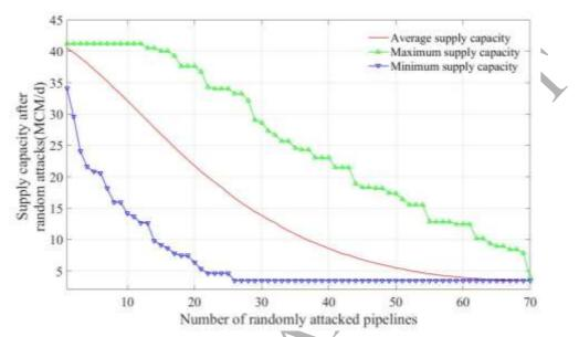
Fig.4. Results of global vulnerability analysis in terms of system supply capacity
