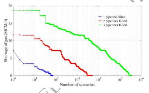
Fig.14. Distribution of shortage for N-1, N-2, N-3 simultaneous failures
