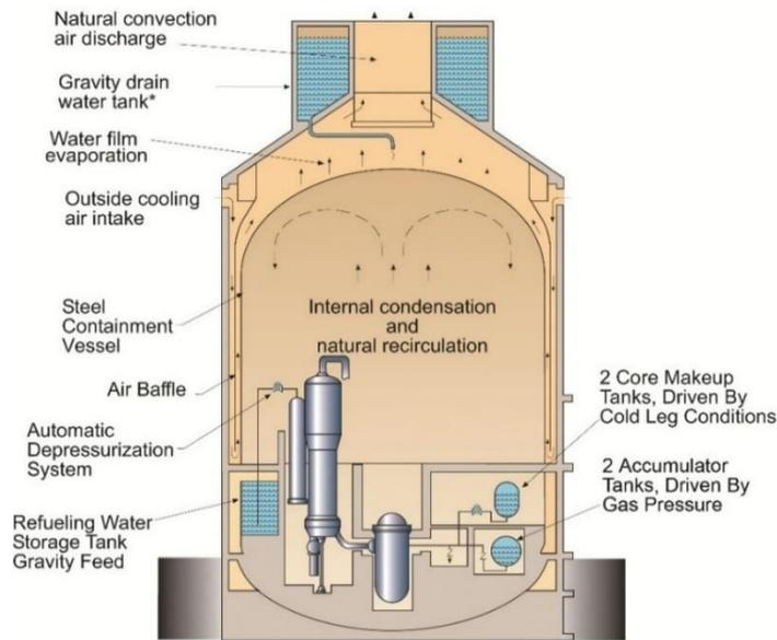
**Fig. 1** An AP1000 Passive Containment Cooling System.
