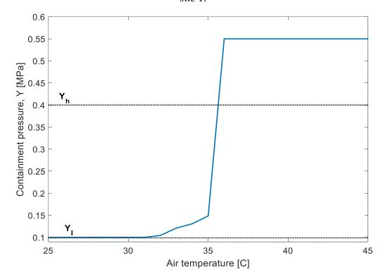
Fig. 17 The critical temperatures leading to the 95th percentile of Y exceeding the safety limit for site 11.
