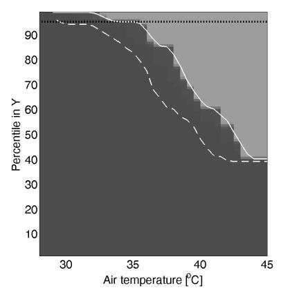
Fig. 15. Profiles of T-Y: probability distributions of Y conditional on T with the percentiles for two critical pressures  $Y \le 0.10$  MPa (dashed white) and  $Y \ge 0.4$  MPa (solid white).
