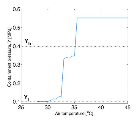
Fig. 16 The critical temperatures leading to the 95th percentile of Y exceeding the safety limit for site 1.
