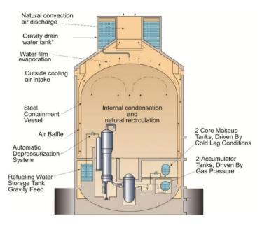
Fig. 1 An AP1000 Passive Containment Cooling System.
