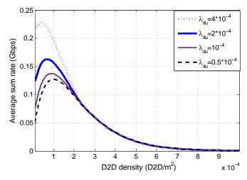
Figure 6: Average sum-rate vs. D2D density (number of D2D pairs per m<sup>2</sup>).
