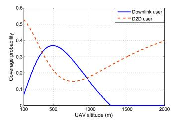
Figure 8: Coverage probability vs. UAV altitude.
